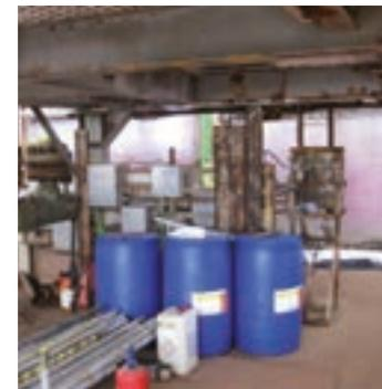
The main risk associated with topsides removal is that the topside is not properly prepared as per the pre-agreed interface matrix, that liquids are left behind without proper identification so that contractors have no idea what they deal with, or that preparatory works have been done differently to that agreed in the engineering phase without informing the contractor. The consequence of these can be substantial and may require costly re-work by the HLV contractor with its crane vessel on site.
